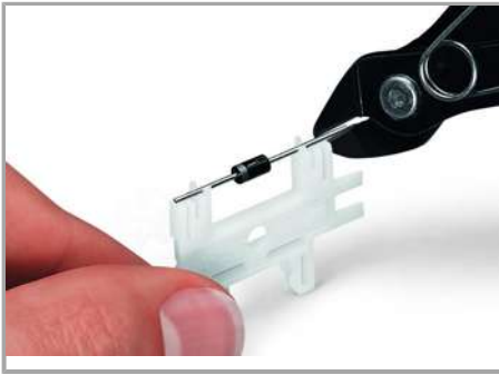
Cutting component to the proper length.
