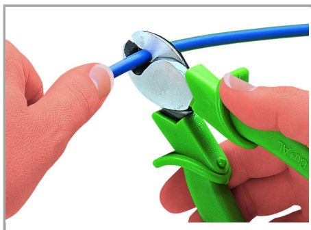
Cutting a cable.
