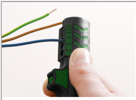
Stripping a wire insulation.
