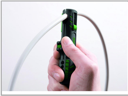
Sheath stripping: longitudinal cut
