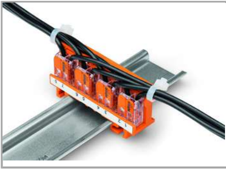
Strain relief via cable ties on the mounting carrier (transverse to the connectors' wiring direction) – clamping units labeled via marking strips (210-334).
