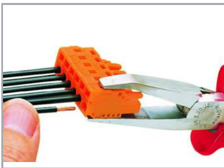
Inserting a conductor via operating tool.
