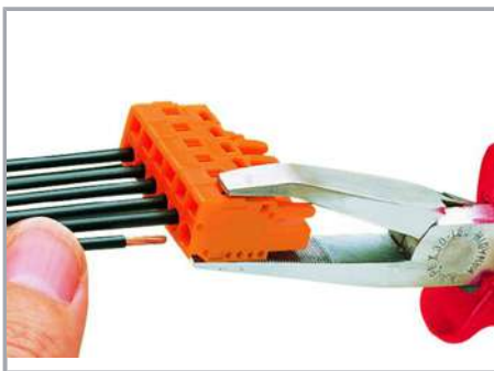
Inserting a conductor via operating tool.
