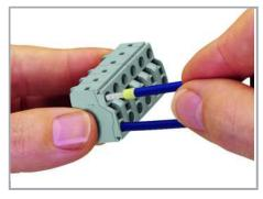
Solid conductors  $\geq$  0.5 mm² (20 AWG), as well as ferruled, fine-stranded conductors can be terminated by simply pushing them into unit. Integrated test ports allow touch contact with current bar via test probes in both horizontal and vertical directions.
