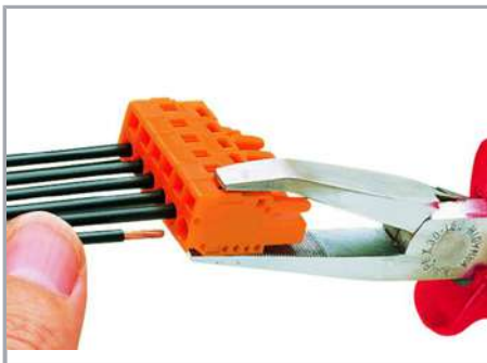
Inserting a conductor via operating tool.
