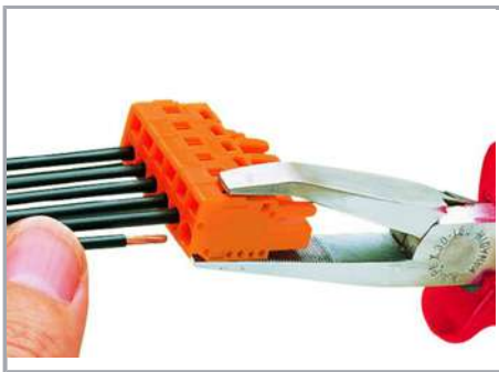
Inserting a conductor via operating tool.
