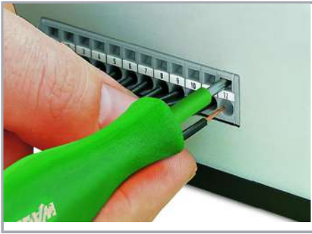
Feedthrough PCB terminal strips – front-entry conductor termination
