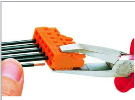
Inserting a conductor via operating tool.
