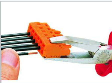
Inserting a conductor via operating tool.
