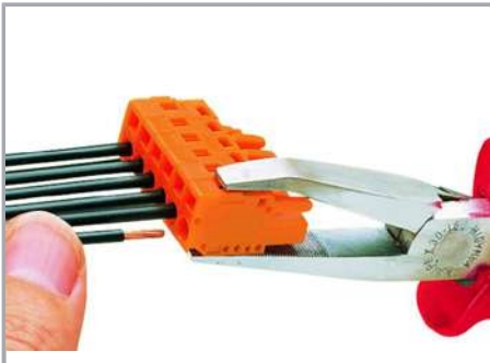
Inserting a conductor via operating tool.
