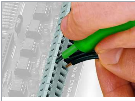
Inserting a conductor via 3.5 mm screwdriver.
