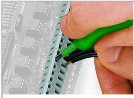
Inserting a conductor via 3.5 mm screwdriver.
