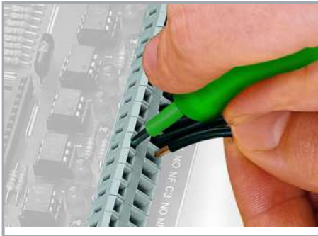
Inserting a conductor via 3.5 mm screwdriver.
