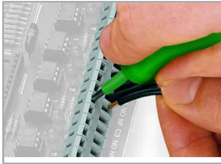
Inserting a conductor via 3.5 mm screwdriver.
