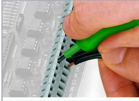
Inserting a conductor via 3.5 mm screwdriver.
