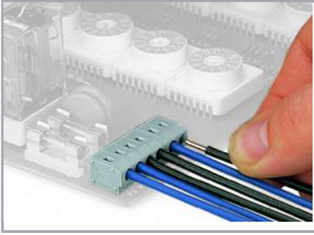
Inserting a solid conductor via push-in termination.
