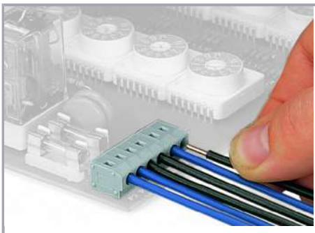
Inserting a solid conductor via push-in termination.
