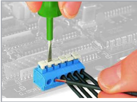
Inserting/removing fine-stranded conductors via push-button.
