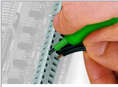
Inserting a conductor via 3.5 mm screwdriver.
