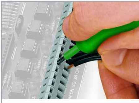
Inserting a conductor via 3.5 mm screwdriver.
