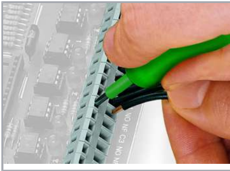
Inserting a conductor via 3.5 mm screwdriver.
