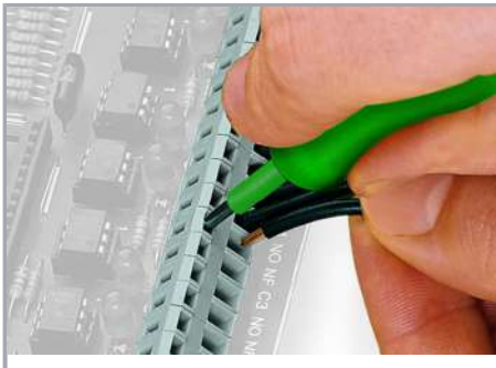
Inserting a conductor via 3.5 mm screwdriver.
