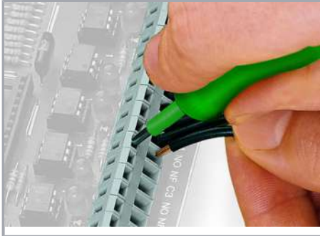
Inserting a conductor via 3.5 mm screwdriver.
