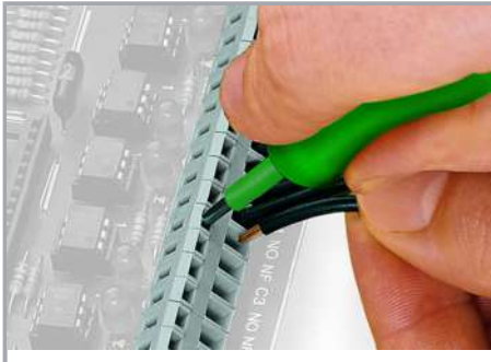
Inserting a conductor via 3.5 mm screwdriver.
