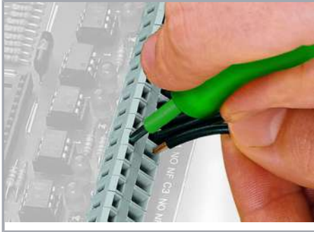
Inserting a conductor via 3.5 mm screwdriver.
