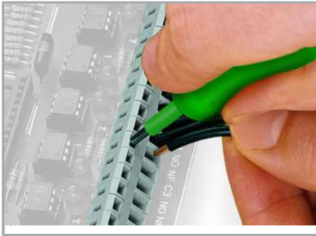
Inserting a conductor via 3.5 mm screwdriver.
