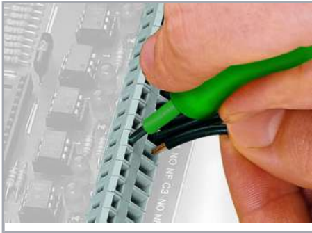
Inserting a conductor via 3.5 mm screwdriver.
