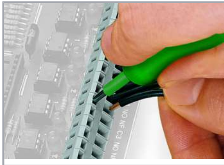
Inserting a conductor via 3.5 mm screwdriver.
