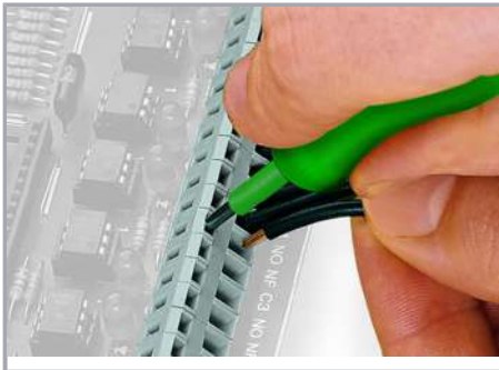
Inserting a conductor via 3.5 mm screwdriver.
