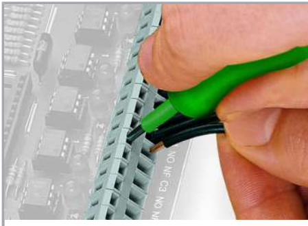
Inserting a conductor via 3.5 mm screwdriver.
