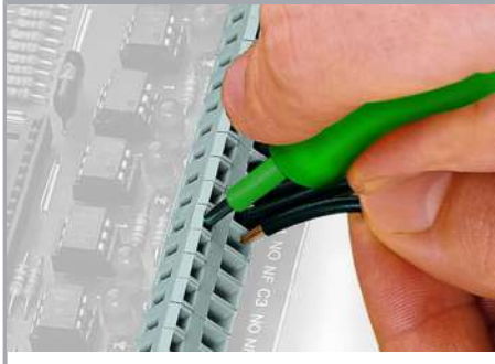
Inserting a conductor via 3.5 mm screwdriver.
