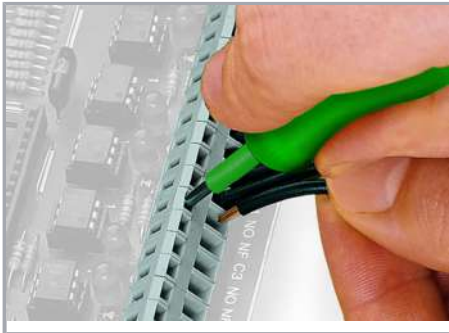
Inserting a conductor via 3.5 mm screwdriver.
