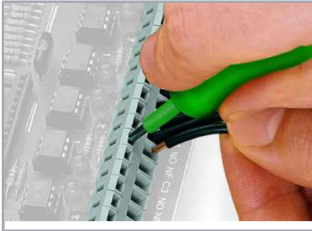
Inserting a conductor via 3.5 mm screwdriver.
