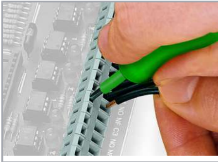
Inserting a conductor via 3.5 mm screwdriver.
