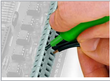
Inserting a conductor via 3.5 mm screwdriver.
