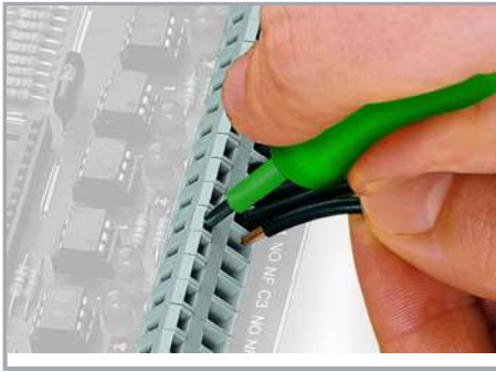
Inserting a conductor via 3.5 mm screwdriver.
