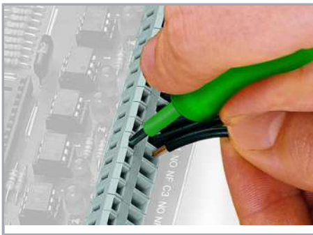
Inserting a conductor via 3.5 mm screwdriver.
