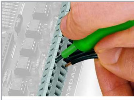
Inserting a conductor via 3.5 mm screwdriver.
