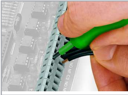
Inserting a conductor via 3.5 mm screwdriver.
