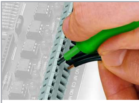
Inserting a conductor via 3.5 mm screwdriver.
