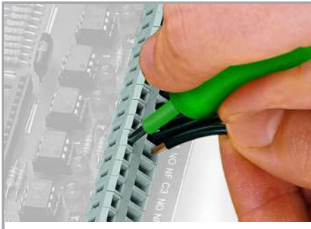
Inserting a conductor via 3.5 mm screwdriver.
