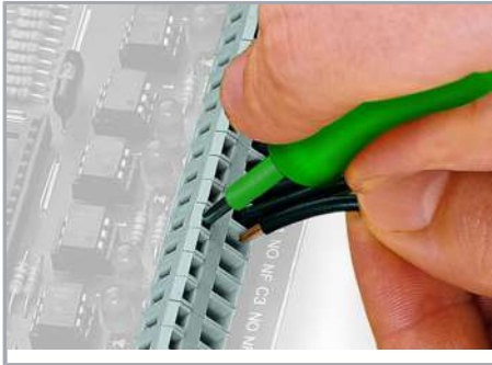
Inserting a conductor via 3.5 mm screwdriver.
