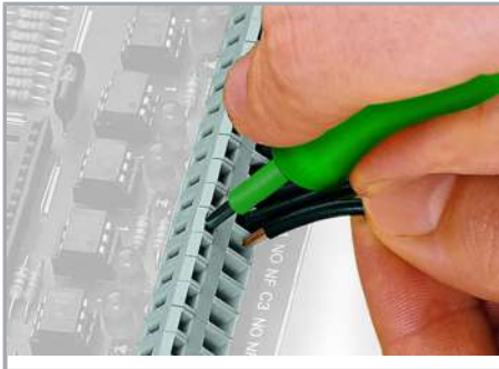
Inserting a conductor via 3.5 mm screwdriver.
