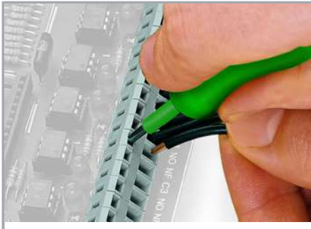
Inserting a conductor via 3.5 mm screwdriver.
