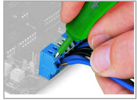
Removing a conductor.
