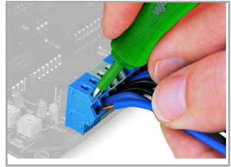
Removing a conductor.
