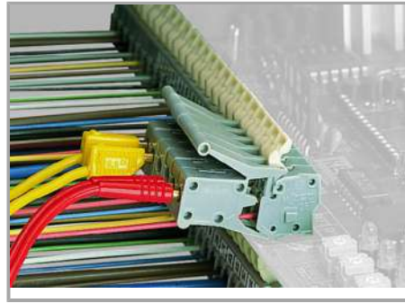
Testing with test plug modules.
